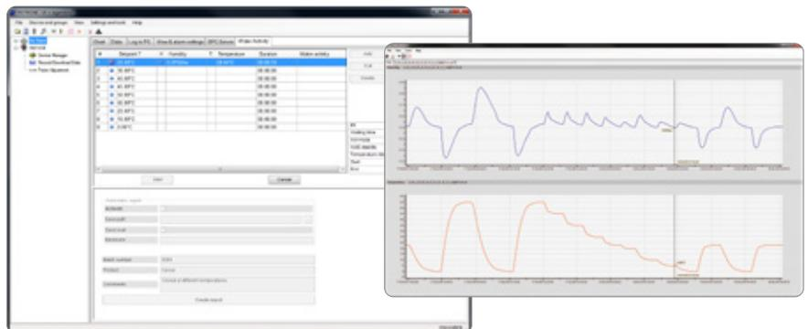
Fully automatic aw measurement can be planned if the AwTherm is connected to the HW4 software. The instrument then moves to preset temperature points automatically and carries out a pre-selected Aw Quick or Aw Equilibrium measurement.
