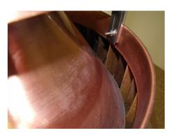
FEATURES: Dividing cup made in a single piece from die for better accuracy.
