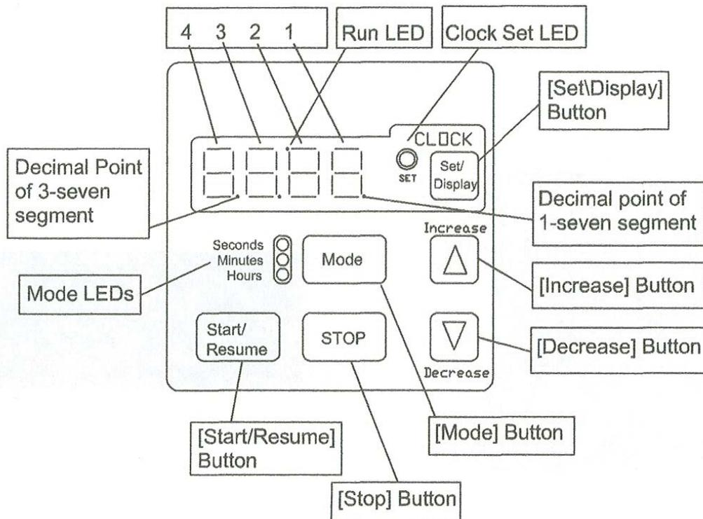
1. After applying an appropriate AC to the power input terminals, the display will be blank and the beeper will beep for  $\frac{1}{4}$  second giving the user notification that the timer is now activated. The units' default is in Minute [Mode].
