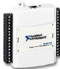
The **NI USB 9211A** Windows Based DAQ for Thermocouples and the **NI USB 6008 Multi function DAQ**, are modular bus powered data acquisition modules that convert the analogue data from the sensors in to 0-20 ma linear output, or low voltage signals.
