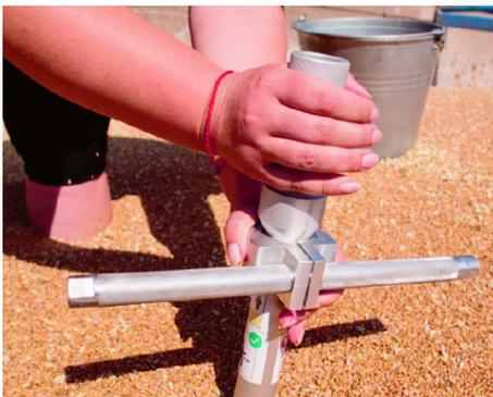
The lightweight aluminium construction means even the long samplers are easy to operate and handle. The tip is fixed permanently so it can not be lost.
