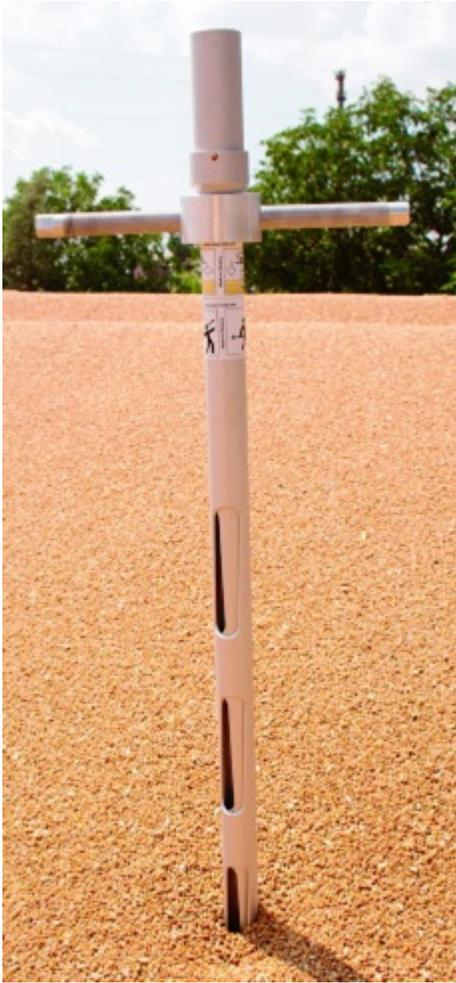
Highly representative sampling is fast and simple with our aluminium grain Spear sampler. This spiral sampler is easy to use and gives great results.
