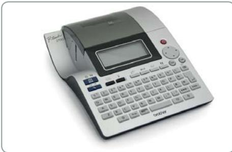
Produce your own etching masks quickly and easily. Simply type the text you require and print it straight on to the etching paper. The etching paper is supplied in a special cassette
