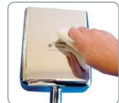
4. Clean etching area thoroughly using demineralised water
