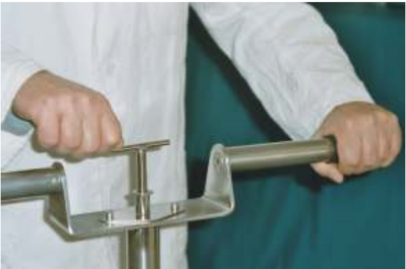
Control to open the sampler
