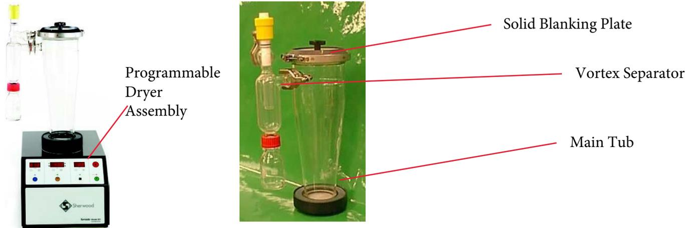
The vertical chamber (tub) is designed to allow air in at the bottom and flow upwards. Air flow out the top of the main tub is inhibited by the presence of a solid blanking plate. The side collection vessel has a vortex separator, in which particles flowing from the main tub hit the central tube in the vortex separator and drop to the bottom of the collection vessel.
